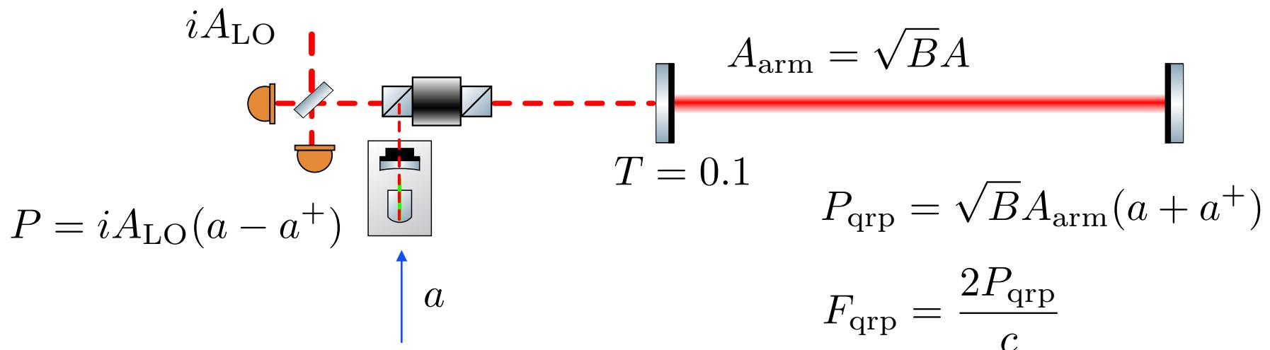
B is the power build-up in the resonator
