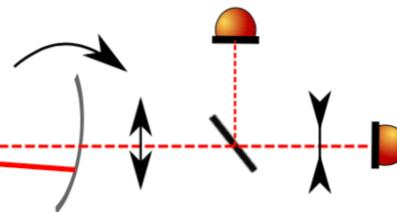
Angular motion is stabilized with bandwidth of 3 Hz.
