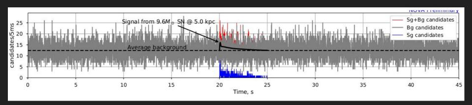
Trigger system needs to distinguish between Bg vs Bg+SN hypotheses.
