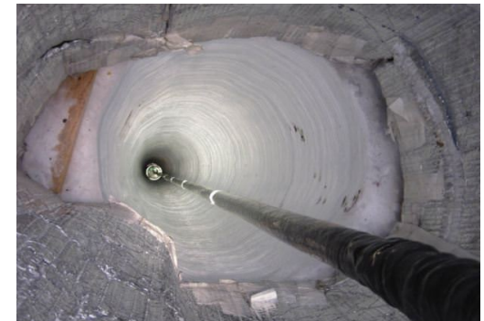
String with optical module
