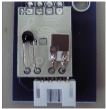
AM2303 \pm 2\% of humidity level \pm 0.3^\circ\text{C} temperature
