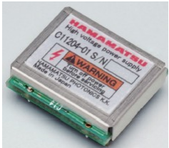
C11204-01 Output Voltage: 50V to 90V
